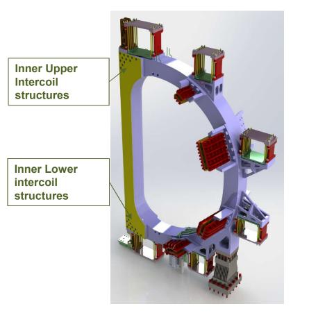
Maintain the connection of the upper and lower part of the TF coil during energization reducing its radial outward movement and minimizing the cyclic loads The system consists in 9 M33 superbolts (460 KN) each side and 3 Superbolt EzFit M33 used as shear pins.
