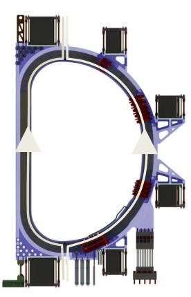
In order to reduce the heat load from the plasma to the WP active cooling system is added to the TF case 4 Channels diam 10mm
