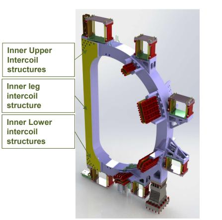
Maintains the connection on the internal straight leg between the TF coils
