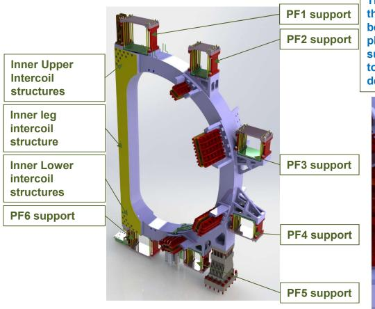
Mantains the PF coils in position supporting their weight (PF1/6 17,8 Ton, PF2/5 18,5, PF3/4 30,9 Ton) and magnetic loads (Max 40MN). The system consists in a cage of 12 rods (diam 24mm) that compress the PF on a sector of about 20° between two steel plates; two G10 sheets (3mm) are placed between the steel and the PF; the cage is supported by two flexible columns that are designed to support the vertical loads and leave the radial deformation free.
