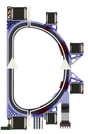
In order to reduce the heat load from the plasma to the WP active cooling system is added to the TF case 4 Channels diam 10mm
