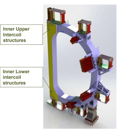
Maintain the connection of the upper and lower part of the TF coil during energization reducing its radial outward movement and minimizing the cyclic loads The system consists in 9 M33 superbolts (460 KN) each side and 3 Superbolt EzFit M33 used as shear pins.
