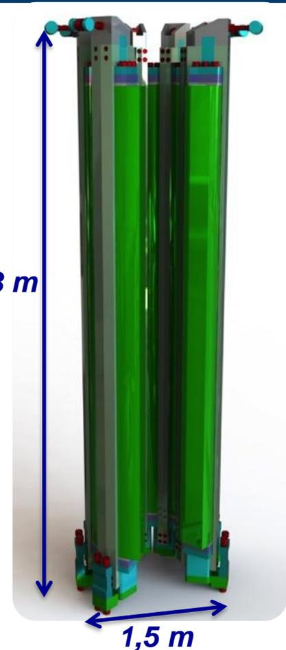
CS pre-assembly to be performed after cold testing at full current
