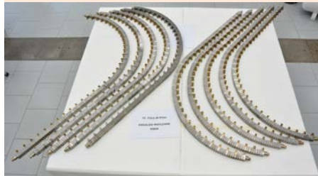
Full scale full W ITER divertor inner vertical target plasma facing units
