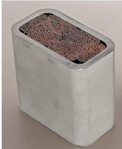
*Figure 4.21: a rectangular CICC conductor solution, with steel jacket of constant thickness [4.2], qualitatively representative of the solution proposed for the DTT CS conductor.*
