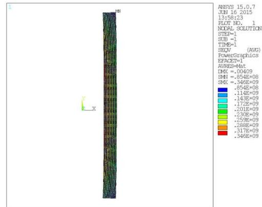
Figure 4.27: SS jacket induced von Mises stress.
