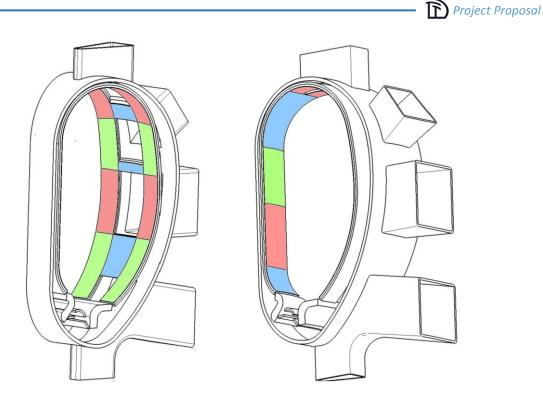
Figure 4.79: Provisional FW segmentation in poloidal plane
