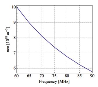
Figure 4.101: Cutoff density in Deuterium plasma when the toroidal phase difference between straps is 180 deg.
