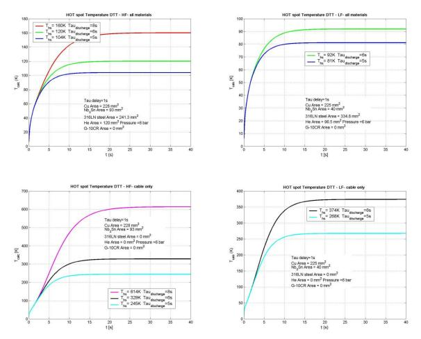
Figure 4.4: upper: (a) Hotspot calculation for DTT TF conductors during a quench, when all conductor materials are considered; results for the HF and for the LF CICCs are shown on the left and on the right, respectively; lower: Hotspot calculation as above, but with only Cu and SC cable content retained.
