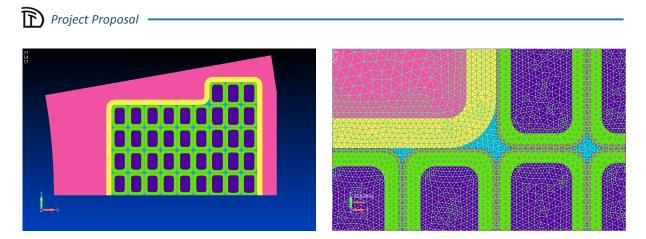
Figure 4.9: 2D model: global view (left), mesh detail (right).
