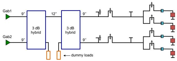
Figure 4.98: Possible upgrade of the matching system, using two 3 dB hybrid couplers.
