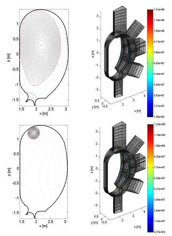
Figure 4.60: Plasma evolution and corresponding eddy currents patterns
