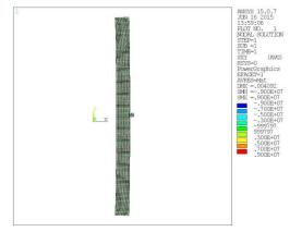
Figure 4.26: Insulation layer induced maximum shear stress area.
