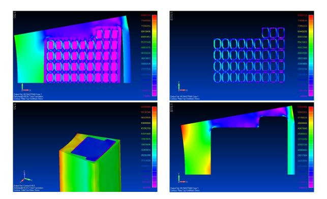
*Figure 4.10. Upper: (2D model) Von Mises stresses global view (left) and on conductor jacket (right). Lower: Von Mises stresses in the TF inner leg at equatorial plane, from 3D (left) and 2D (right) analysis.*
