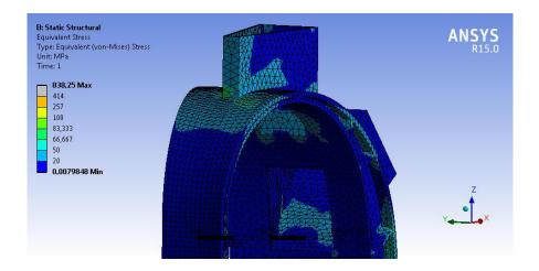
Figure 4.72: Von Mises Stress upper area
