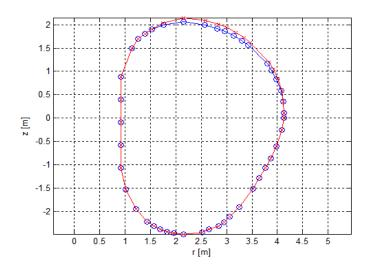
Figure 4.12: Poloidal trace of the TF coil outer surface (farther from the plasma): nominal (blue circles), deformed (red crosses)
