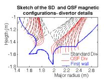
Figure 3.9: Details of the divertor region for the computed equilibria for SD (black) and QSF (red)
