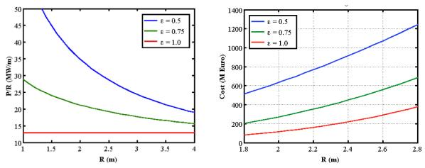
Figure 3.1: Left-P/R scaling versus R for three different  $\varepsilon$  parameters: for  $\varepsilon = 1$  P/R is always too small; Right-Load Assembling device cost; for  $\varepsilon = 0.5$  the cost is always too high.
