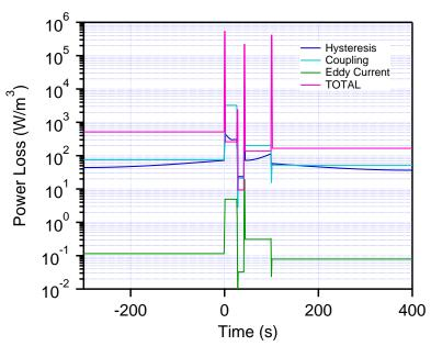
Figure 4.43: Total power loss and contributions due to various mechanisms, vs. time in the pancake subject to the largest field.
