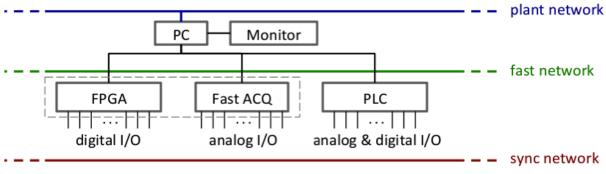
Figure 4.104: Architecture of the CODAC system.
