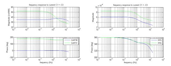
Figure 4.40: Use of in-vessel coils for strike point sweeping: dynamic response of the two strike points to a current flowing C1 and C3 connected in antiseries. The currents induced in PF5 and PF6 are also shown.
