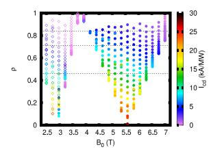
Figure 4.111: Radial locations  $\rho$  that can be reached (vertical axis) at different magnetic field strengths B0, via a poloidal steering of the beam for a toroidal injection angle  $\beta=16^{\circ}$ . The respective driven current  $I_{cd}$  is indicated by the color code. Injection of both O-mode (full circles) and X-mode (open diamonds) is considered.
