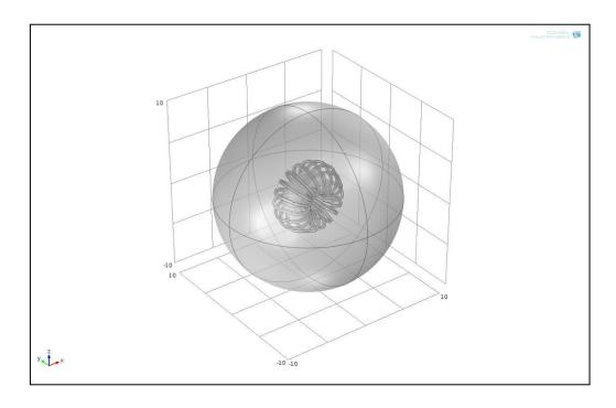
Figure 4.11: 3D view of complete TF coil system with a sphere positioned at origin of coordinate system and having a radius of r = 10 m
