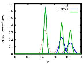
Figure 4.109: Absorbed power density dP/dV for injection from the equatorial (EL) and upper (UL) port, aiming at the q=1, q=3/2, and q=2 surfaces with a toroidal launching angle  $\beta$ =10°. For the equatorial launcher both upwards and downwards injections have been considered, reaching the rational surfaces above and below the equatorial plane respectively.
