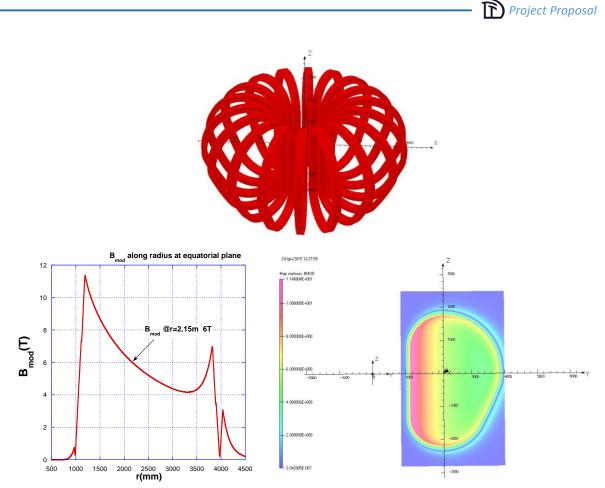
Figure 4.5: upper: 3D model used for simulations; lower: Bmod(r) at equatorial plane (left); B map over the TF coil vertical section (right)
