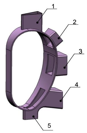
*Figure 4.46: DTT VV – 20° module with ports provisional numbering*
