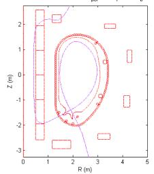
Figure 4.35: Reference SN scenario: magnetic configurations.
