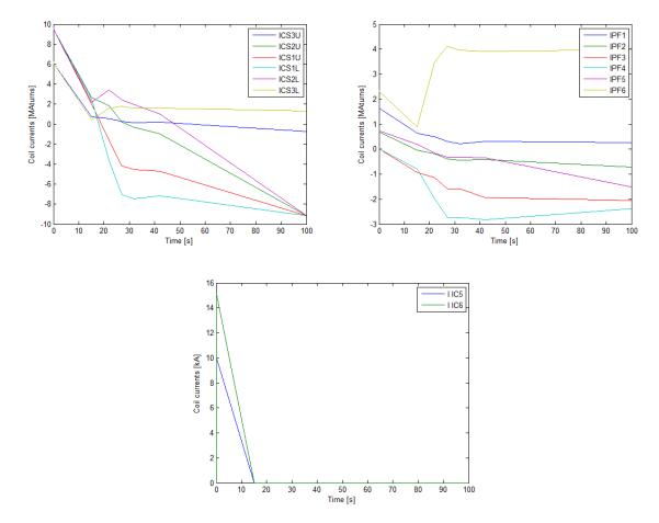
Figure 4.33: Reference SN scenario: coil currents.
