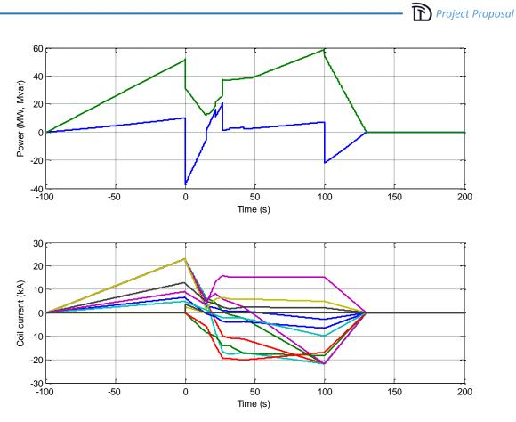
Figure 4.135: Relationship between electric power and current scenario for poloidal coils.
