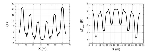
Figure 4.6: Magnetic field as a function of the hydraulic length of the HF conductor
