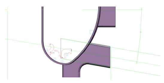
Figure 4.48: Port nr. 4 is arranged to ease the access to divertor
