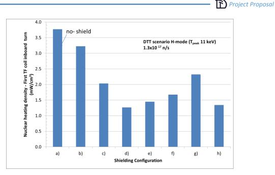
Figure 4.84: Nuclear heating density of the first TF coil inboard turn for different shielding configurations
