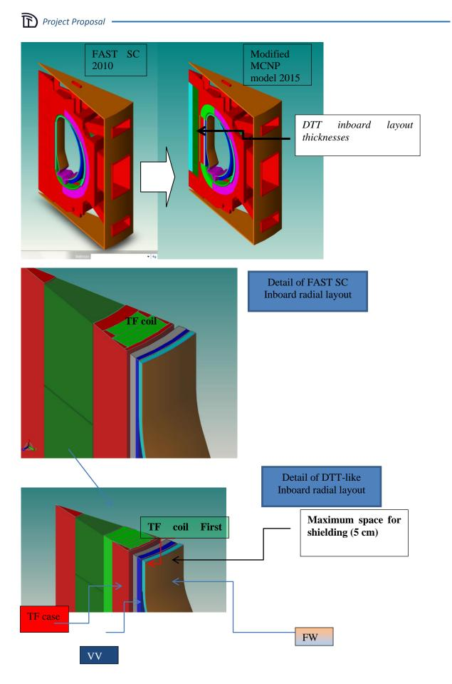
Figure 4.83: Modified MCNP model of FAST used for this pre-assessment and comparison with FAST SC 2010
