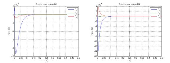
Figure 4.56: Forces acting on the vessel (material #1) and port extension #3 (material #4)
