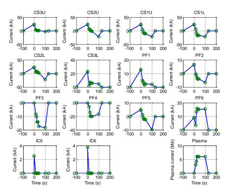
Figure 4.130: Current scenario for each magnetic coil.
