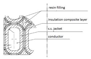
Figure 4.24: Schematic of the conductor section.
