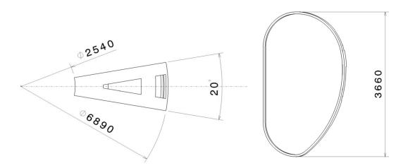
Figure 4.45: Overall dimensions (in mm) of main vessel sector (top and side views)
