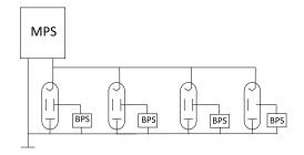
Figure 4.117: Scheme of a single MPS module feeding 4 gyrotrons
