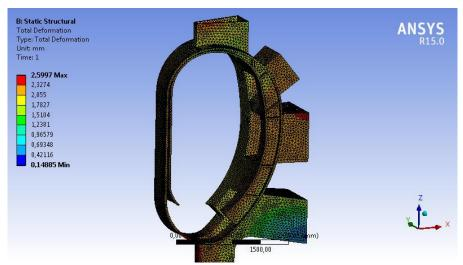
Figure 4.75: DTT Vessel total displacement
