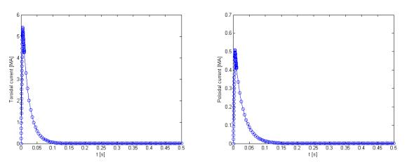
Figure 4.55: Total toroidal and poloidal current induced in the structures (except the PF coils)
