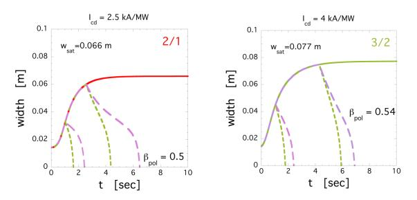
Figure 4.112: Time evolution of the island width computed from the Generalised Rutherford Equation. The green dashed lines refer to  $w_{cd} = 4$  cm and the violet to  $w_{cd} = 5$  cm. The width  $w_d = 3$  cm. Left: 2/1 mode; right: 3/2 mode.
