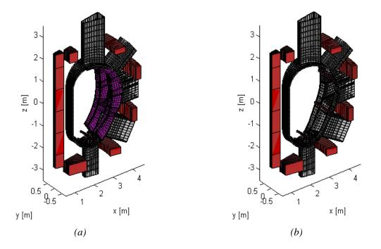
Figure 4.58: Discretizations used for self-consistent disruption analysis.
