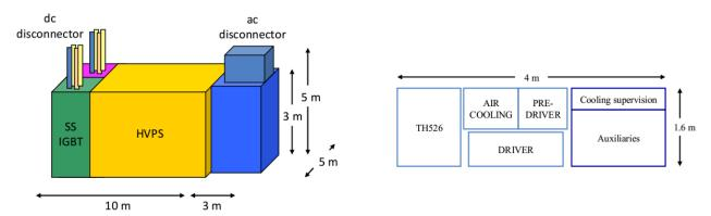
Figure 4.105: Single module of HVPS (left) and single amplification chain (right).
