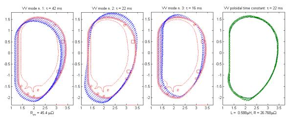
Figure 4.148: L/R time constant of DTT vacuum vessel, consisting in a single 35 mm shell of INCONEL: 1) 42 ms for magnetic flux (and toroidal electric field) penetration; 2) 42 ms for radial magnetic field penetration; 3) 16 ms for vertical magnetic field penetration; 4) 22 ms for toroidal magnetic field penetration.
