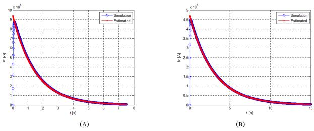
Figure 4.64: Poloidal current induced in the vessel by a TF discharge: (a)  $\tau_D = 1.5 \text{ s}$ ; (b)  $\tau_D = 3 \text{ s}$ .
