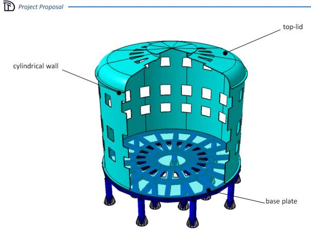
Figure 4.126: Cryostat Vessel segmentation
