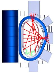
*Figure 4.144: Overview of interferometer-polarimeter* 6+5 *viewing chords.*
