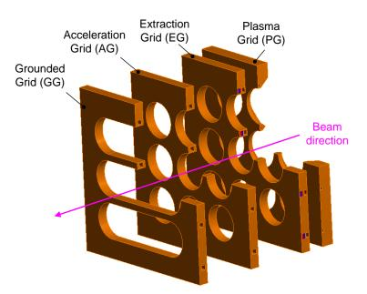
Figure 4.122: acceleration stages concept
