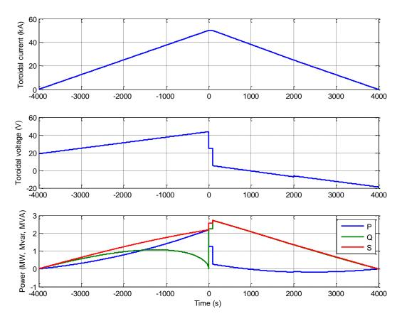
Figure 4.136: Current, voltage and electric powers for toroidal coils.
