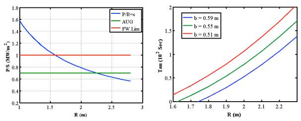
Figure 3.2 Left: Power density, versus the machine radius, assuming P/R=Cost=15MW/m, Right; Discharge duration, versus the machine radius, at different central solenoid width
