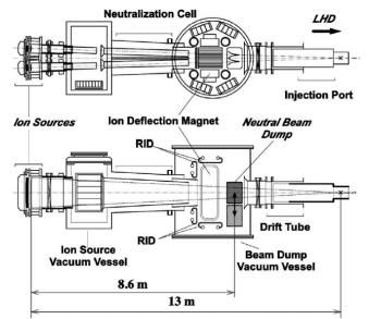
Figure 4.121: LHD Negative Neutral Beam injector. Similar layout is proposed for DTT. The same layout is also adopted in JT-60SA.
