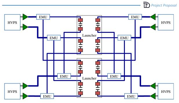
Figure 4.99: Feeding scheme of the straps of two launchers with eight external matching units (EMU).
