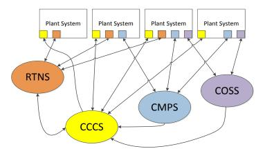
Collectively DICS perform a number of top level DTT functions necessary to manage the experiment (Orchestration and monitoring of Plant systems, control functions, data collection etc). Its functions are implemented by a combination of systems and subsystems (interfaces, networks, monitoring, management etc).
