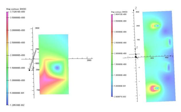
Figure 4.31: Details of magnetic field map at SF+ @SOF for PF1 (left); DN@SOF for PF2,3,4,5 (right).
