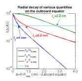
Figure 3.10: e-folding decay lengths
