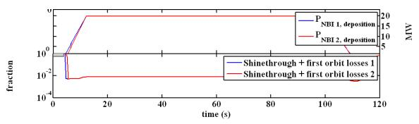
Figure 4.120: NBI power deposition waveform and shinethrough fraction.
