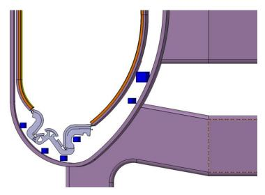
Figure 4.82: A possible DTT divertor for a single null configuration
