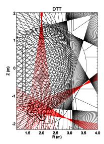
Figure 4.145: Layout of bolometer arrays
