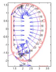
Figure 4.150: Plasma-wall gaps that can be used for plasma shape control.
