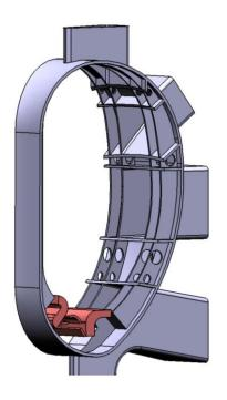
Figure 4.80: Conceptual FW support structure at outboard side of the vacuum chamber
