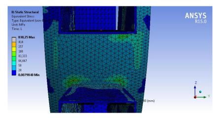
Figure 4.73: Von Mises Stress Lower area
