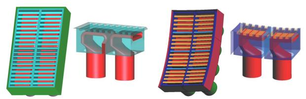
Figure 4.100: Antenna (left) and cutoff density in a Deuterium plasma (right) when the phase difference between the straps of the same row is 180 deg.
