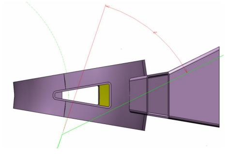
Figure 4.50: Enlarged equatorial port aimed at accommodating the co-tangential NBI beam
