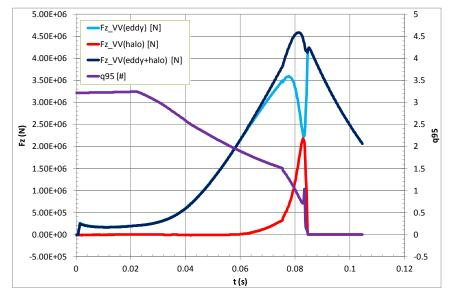
Figure 3.17: Vertical forces on the VV due to the halo and eddy current in the Category IV upward VDE.
