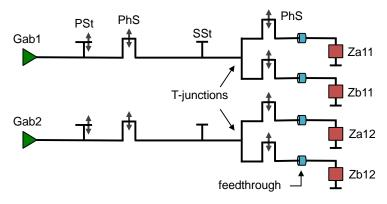
Figure 4.97: External matching system with two conjugate-T, feeding the straps in half a column of two antennas.
