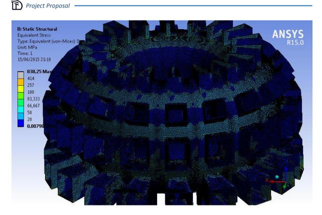
Figure 4.74: Von Mises Stress – Cyclic Symmetry
