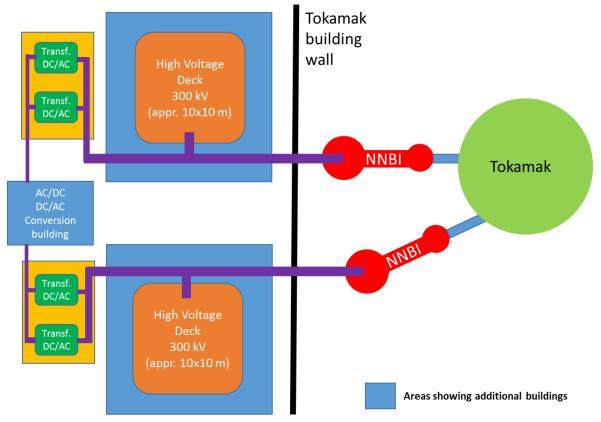
Figure 4.124: Layout of NNBI injector and PS
