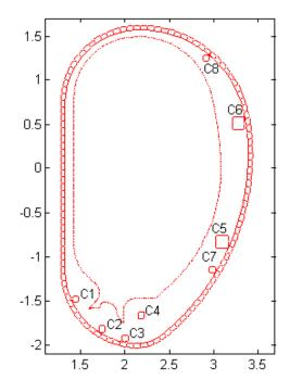
Figure 4.32: In-vessel copper coils.
