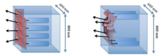
*Figure 4.115: Sketch of the two options for the equatorial launcher, accommodating up to 4 beam lines. Left: toroidal steering option; right: poloidal steering option.*
