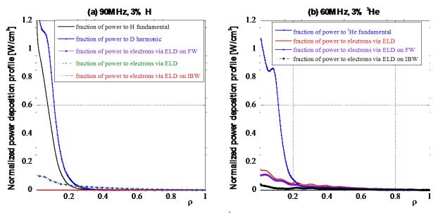
*Figure 4.96: Power deposition profiles [W/cm<sup>3</sup>] normalized to 1 MW of coupled power.*
