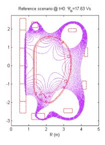
Figure 4.34: Reference SN scenario: pre-magnetization.
