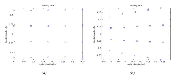
Figure 4.13: Winding pack cross section (18 TF coils case): (a) rectangular, (b) wedge.
