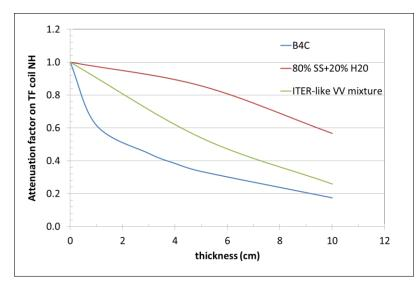
Figure 4.85: Attenuation factor of TF coil nuclear heating (first turn) vs. thickness of additional shielding of  $B_4C$ , 80% SS-316+ 20%  $H_20$  and ITER-like VV mixture.
