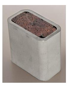
Figure 4.21: a rectangular CICC conductor solution, with steel jacket of constant thickness [4.2], qualitatively representative of the solution proposed for the DTT CS conductor.
