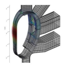
y [m] Figure 4.53: 3D mesh used in the disruption analysis
