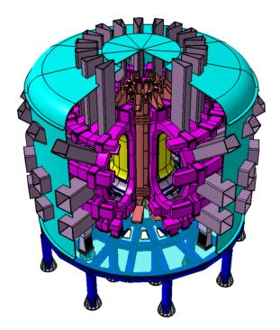
Figure 4.125: Sectional view of DTT tokamak basic machine
