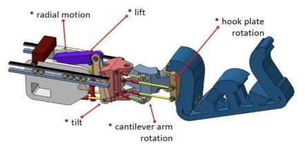
Figure 4.86: Schematic view of the Divertor remote handling system
