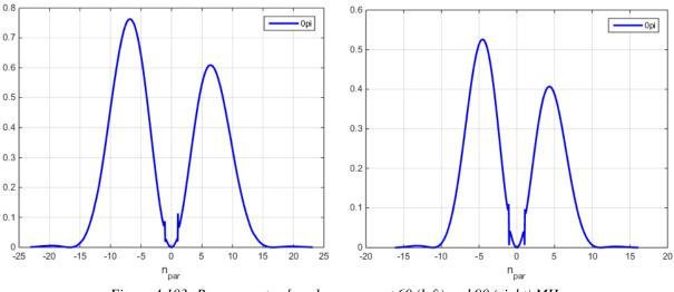
*Figure 4.103: Power spectra [a.u.] versus*  $n_{\parallel}$  *at 60 (left) and 90 (right) MHz.*
