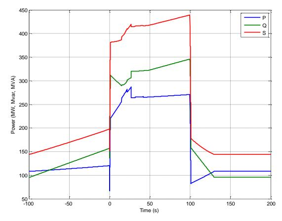
Figure 4.138: Total electric powers for DTT machine.
