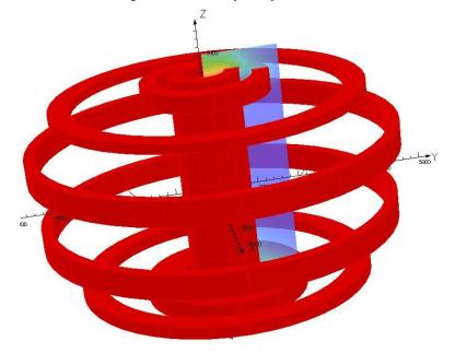
Figure 4.28: Poloidal coil system model
