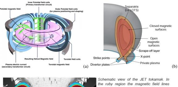
Schematic view of the JET tokamak. In the ruby region the magnetic field lines form concentric nested magnetic surface. The plasma periphery is the yellow region that is just within the last closed magnetic surface (the separatrix). The scrape-off layer (SOL) is the blue region, where the field lines are not closed but end on the divertor plates along an inner and an outer leg (courtesy JET-EUROfusion).
