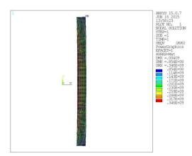
Figure 4.27: SS jacket induced von Mises stress.
