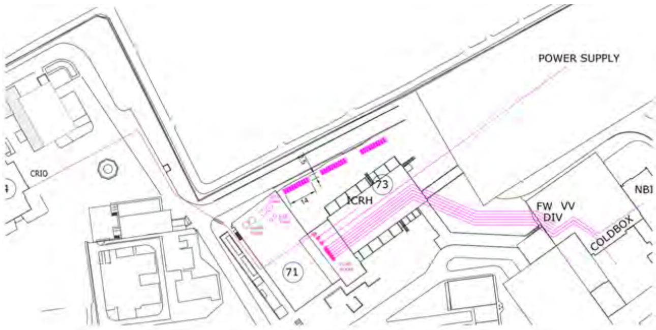
Figure V.7: Layout of the water-cooling system secondary loop.
